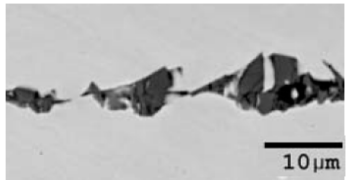
Image 4. BEI of typical over median size inclusion feature in standard ASTM F 562 material.
